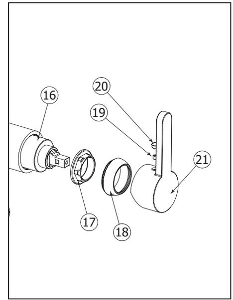
To replace the cartridge, start by shutting off water supply lines and then turn the water on to drain the faucet.
