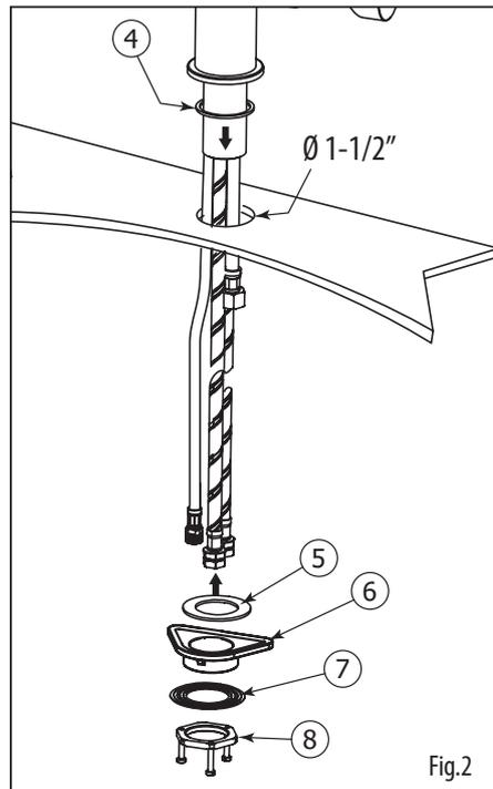
**⚠ WE RECOMMEND DRILLING A 1-1/2" DIAMETER HOLE FOR THE INSERTION OF THE FAUCET.**
