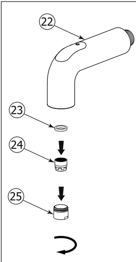
To clean the aerator (24), remove the spray head (22) from the faucet body. Then, using an adjustable wrench, remove retainer ring (25) from its spray head. Extract the aerator (24) and washer (23). Soak the aerator in a vinegar and water solution to remove lime build-up. Once parts have been cleaned, reassemble by reversing steps.
