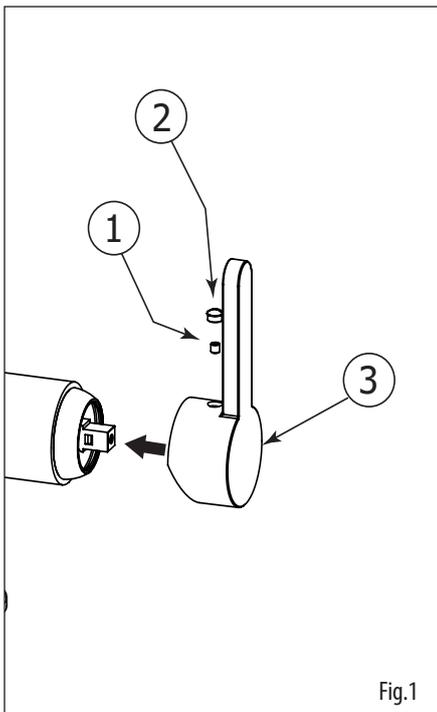
Install the handle (3) by sliding it onto the cartridge broach. Secure it with set screw (1) and cover with aesthetic cap (2).
