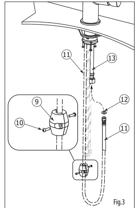
Connect the spray head hose inlet (11) with the mixed water outlet (13). Do not forget the supplied washer (12).
